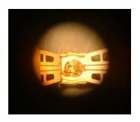
Two IZI-Probes Z040-K3N-GSG 750 were calibrated using CSR-11. The DUT was lying on a plastic surface without any attachment and was directly connected at its solder pads. 5 samples were tested.
