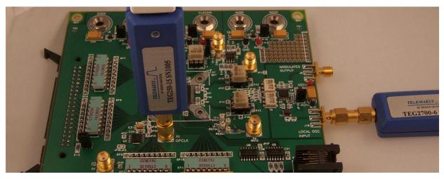
The small size of the TEG devices allow them to be directly connected to the Evaluation board
