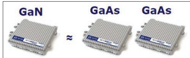
▲ Fig. 1 One GaN amplifier replaces two GaAs amplifiers in analog video, mixed signal and all digital wireline networks.
